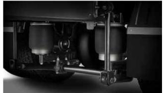
The newly developed rear air suspension is developed for the 4x2 and 6x2 models. In addition to the unique driving comfort, it guarantees much safer transport of fragile loads.
