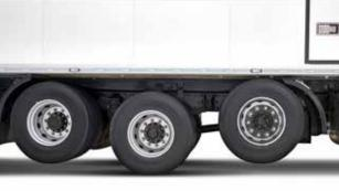
For vehicles with 6x2 and 8x2 axle type, in unloaded conditions, the rear axle is off the ground.
