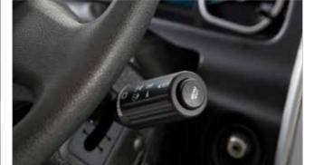
The 600 KW Intarder, which is available as an optional feature on vehicles, meets all expectations under such challenging conditions as going downhill while loaded. Preventing unnecessary use of your service brake, it prolongs service life.
